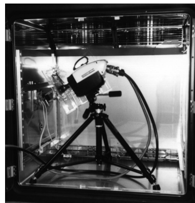
Fig. 7: Setup with high-speed camera in climate chamber allowing particle actuation to be recorded by high speed camera at inclinations up to 90°.
