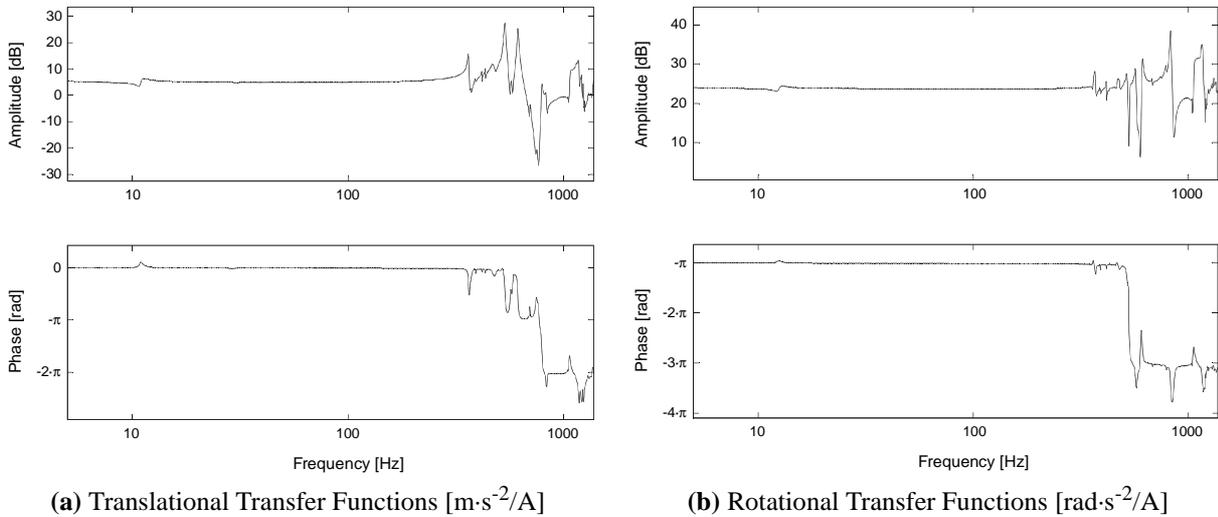
**FIGURE 6:** Typical Transfer Function of one Voice Coil
