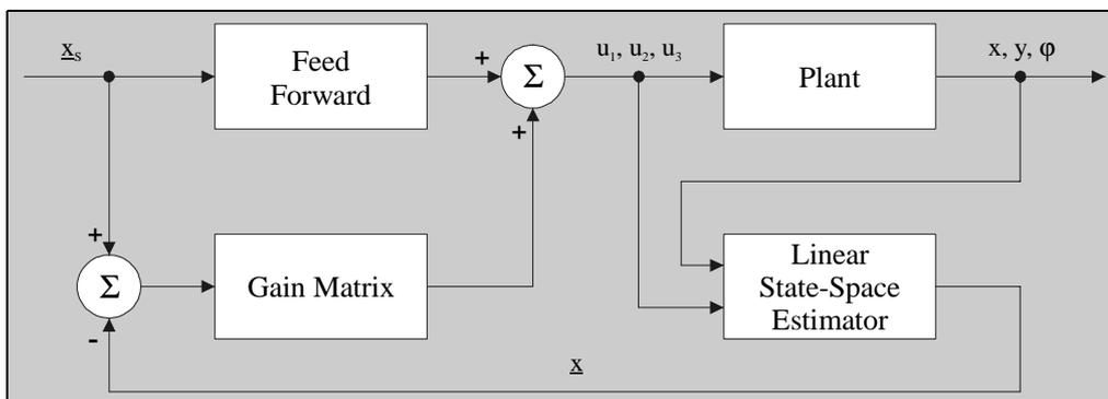
**FIGURE 7:** Linear State-Space Controller with Feed-Forward Path
