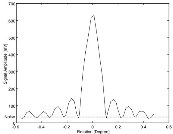
**FIGURE 5:** Amplitude-Rotation Sensitivity
