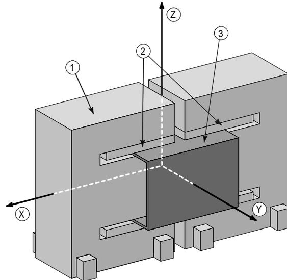
**FIGURE 1:** Voice-Coil Type Actuator (1-Core/Stator, 2-Magnet, 3-Moving Coil)
