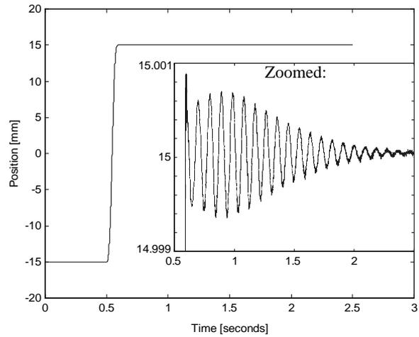
**FIGURE 8:** Fast Movements (30 mm in 90 ms)
