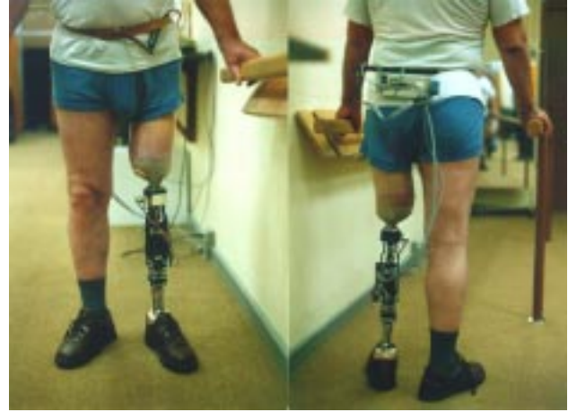
Figure 4: The laboratory prototype of a controlled A/K prosthesis used by a patient in the clinic
